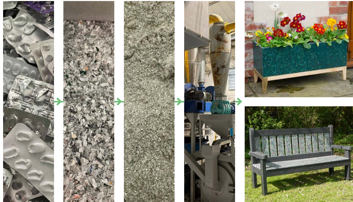
Blister packs are recycled to manufacture new products and support educating children on sustainability.
